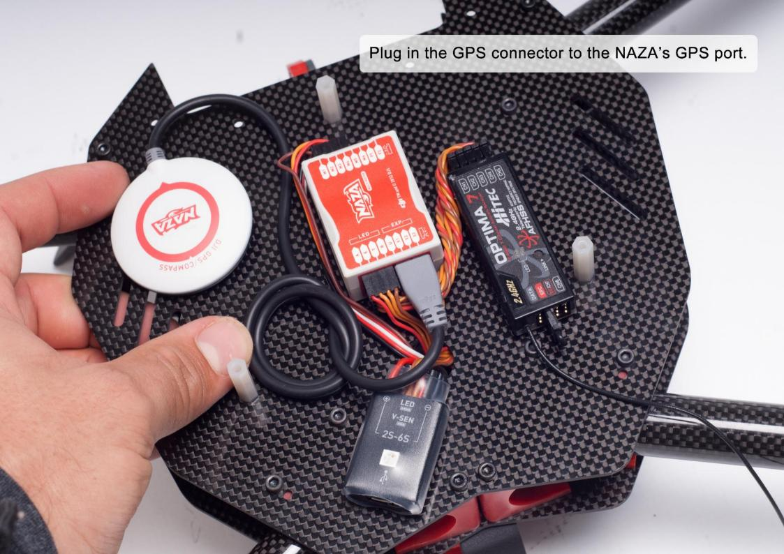
For a neat installation we use the included double side tape for the Naza GPS and stick it directly to the top dome of the QU4D.
