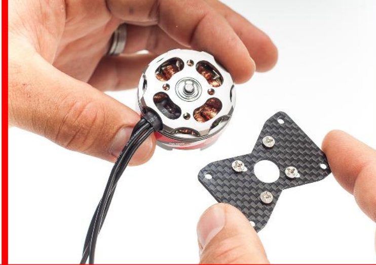
Insert the 4 x 40mm Cap Screws
