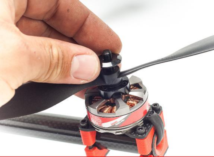
Attach the prop, washer and nut as shown
