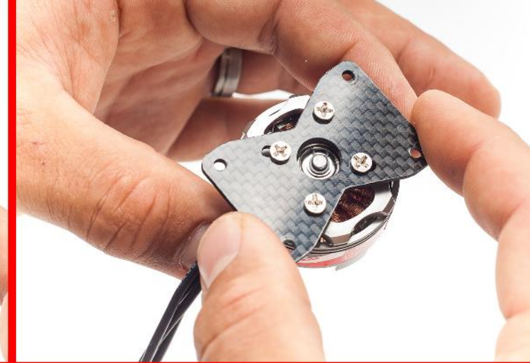
On the side of the motor wires add the spacer plate to tilt the motor inwards
