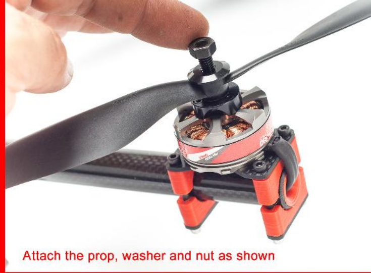
Tighten with a 10mm spanner or socket
