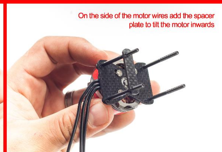
Insert the 4 x 40mm Cap Screws
